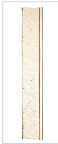
Induro™ FRP wall panel - nominal damage.
